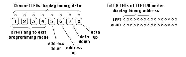
The left 8 LEDs of the left channel VU meter display a binary memory address--LED off=0, LED on =1. When you first enter programming mode, the address will be 27 (00011011 on the VU display). Press the channel 5 button three times to decrement the address to 24 (00011000 on the VU display). Location 24 stores silence sensor link control data.
